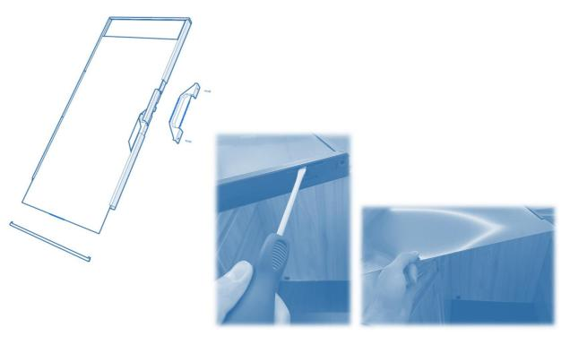
When the magnetic foil has been applied, then the end pieces can be reattached and the door can be hung in the refrigerator front.
