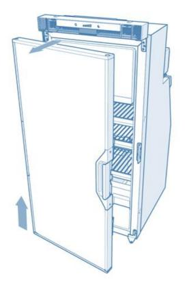
In the case of a refrigerator front with shell handle, optionally, if necessary, the shell handle can be removed.
