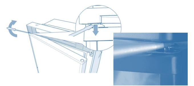
After the connecting bolt has been pressed down, the refrigerator front can be removed.
