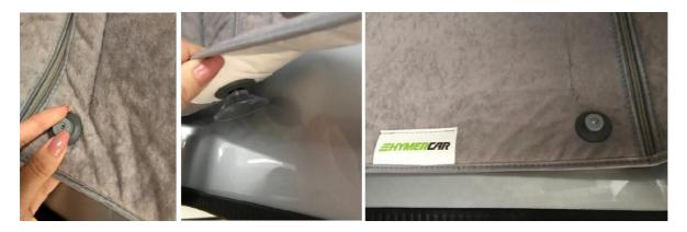
First start by assembling the front section. To do so hold the front part against the front wall and align it centrally. Then attach the front parts at the bottom with the aid of the suction cups. Then mark the points where the lower part of the magnets need to be installed. Now screw the magnets at the top under the roof. Here, the opening of the magnets must point upwards.
