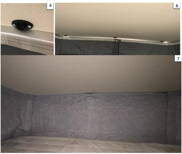
In order to assemble the side sections on the right and left side, first connect the respective side section with the rear and front section. Now assemble the lower magnet parts as before. After this the side parts can simply be attached using the magnets.
