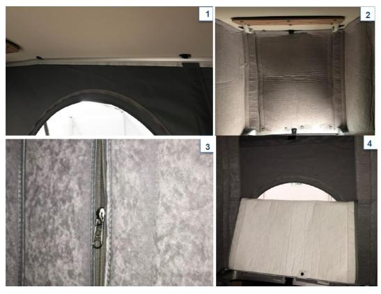
The rear section is installed next. To do so, hold the insulation onto the rear wall and mark the position of the lower magnet parts. Now screw the lower manget parts under the roof. Here also, the openings of the magnets need to point upwards. As soon as all three lower magnet parts are attached, the insulation can be installed.
