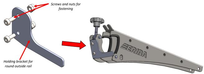
Attach the clothes line holder so that the holding bracket for the round outside rail can be supported by the connector for the round outside rail (on the caravan side).
