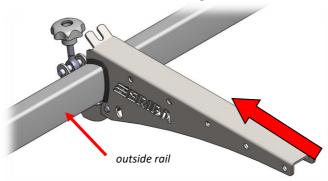
First, swing the bracket upwards and then fit the star handle into the groove.
