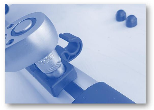
After the covers have been removed, the cap nuts can be loosened with the hexagonal ratchet.
