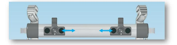
If they do not match, the hook brackets can be adjusted at the base support. Here, the plastic covers would have to be removed (4x in total).
