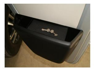
The safe is screwed to the door panel via the original screw points.
