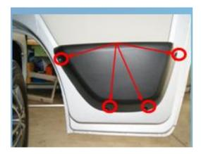
The door storage compartment must be removed in order to be able to install the door safe. In order to do so, the 4 Torx screws must be undone and removed.
