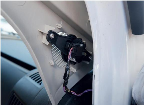
*Carefully remove the A-pillar cladding, place it on the dashboard (protect the surface with adhesive tape), and unclip then unplug the existing original tweeter.*
