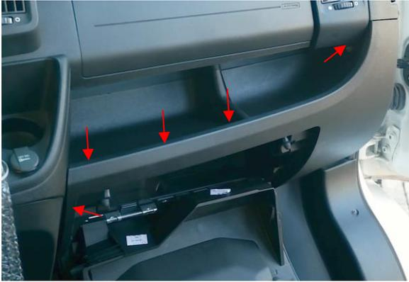
Remove the screw on the inside left under the glove compartment flap, and the screws on the top in the glove compartment cladding.
