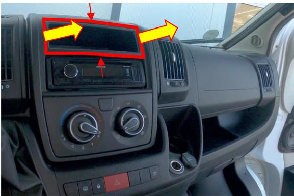
Remove the storage compartment above the radio.
