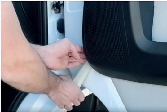
Carefully lift and remove the cover of the woofer using a plastic wedge.
