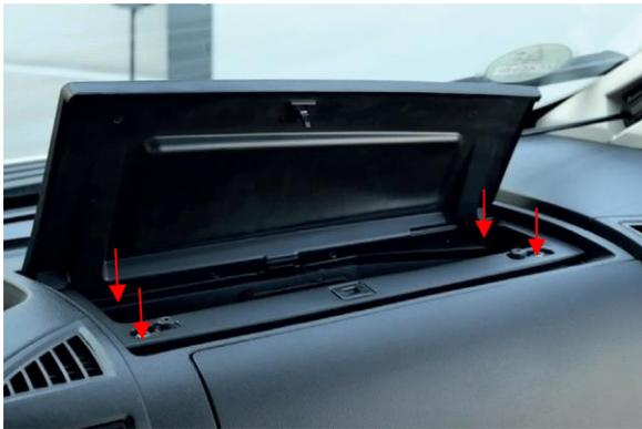
Open the storage compartment, remove the 4 screws inside and put them to one side.
