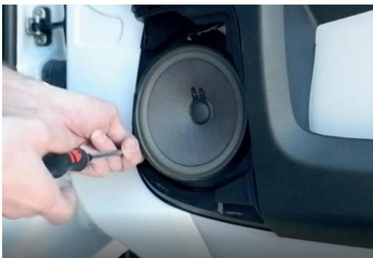
Unscrew and remove the screws for the woofer, and pull out the cable on the casing.
