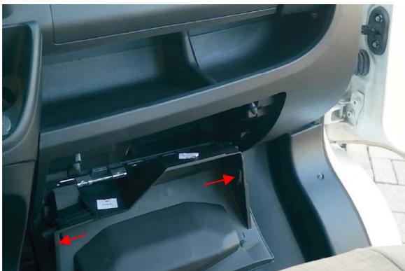
Open the glove compartment and press the clips on the inside to release it so that it can be pulled out completely forwards.
