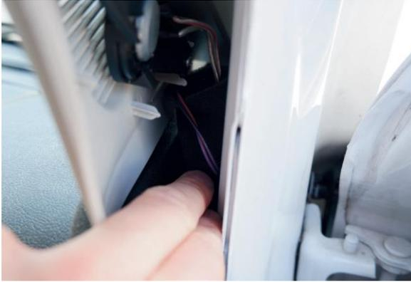
Push the foam sleeve into the area between the dashboard and the A-pillar.
