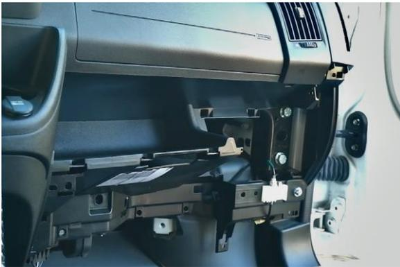
Remove the glove compartment including the cladding part and put it to one side.
