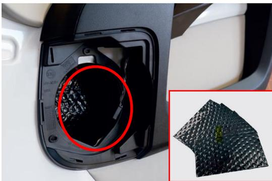
Remove the protective paper from the enclosed Alubutyl sheet, heat it using a hairdryer, and press the butyl side (adhesive) firmly onto the panel behind the woofer opening.
