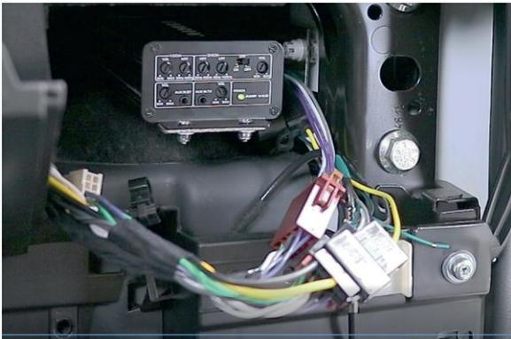
Lay all cables in the space behind the glove compartment.
