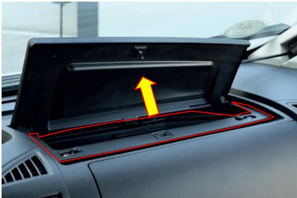
Remove the storage compartment and put it to one side.
