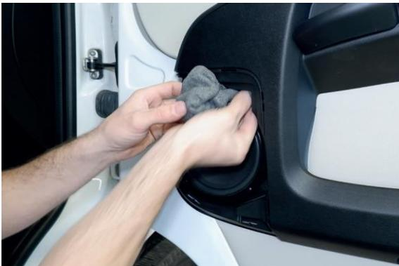
*Slide the foam sleeve over the connection and push it through the opening into the space under the cladding.*
