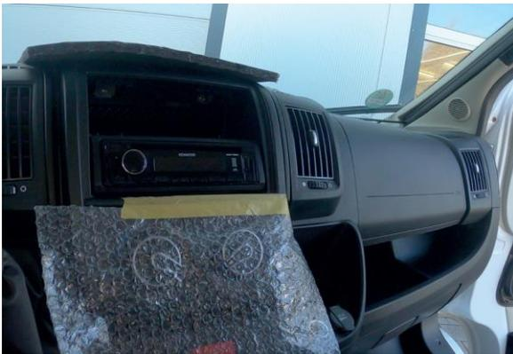
Protect the working area around the radio from damage using suitable material (e.g. masking tape & bubble wrap).
